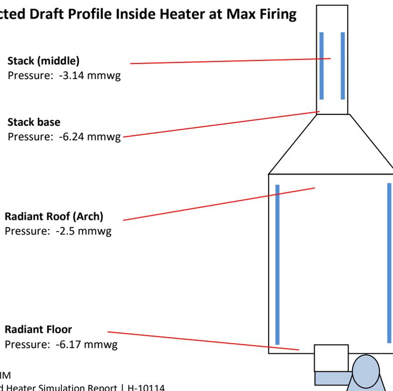
The maximum heat liberation of the burner is 879 kW. The simulation were also carried out at max burner firing rate (please see results attached for full details).
